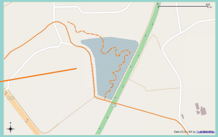
Controlled flooding basin in Bernissem (Sint-Truiden, Belgium)
